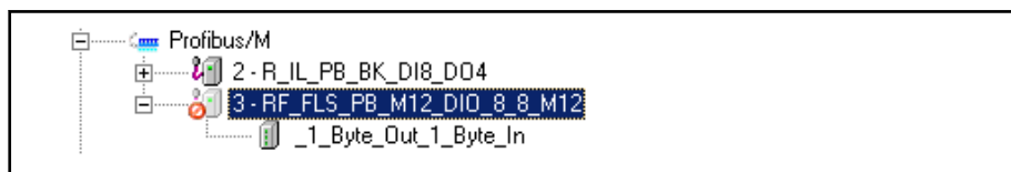
Fig.3-22: PROFIBUS DP with disabled modules
